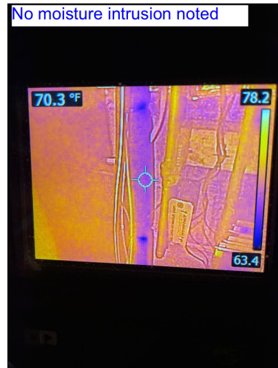
Infrared Meter Scan of Representative Area of Internal Foundation Walls
