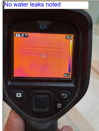
Infrared Meter Scan of Bathroom Shower Basin Area
