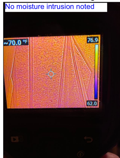
Infrared Meter Scan of Representative Area of Roof Sheathing
