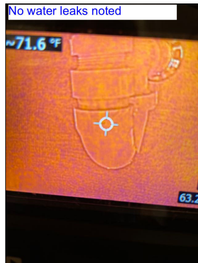
Infrared Meter Scan of Bathroom Trap
