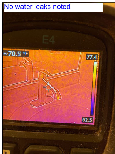
Infrared Meter Scan of Bathroom Sink Area
